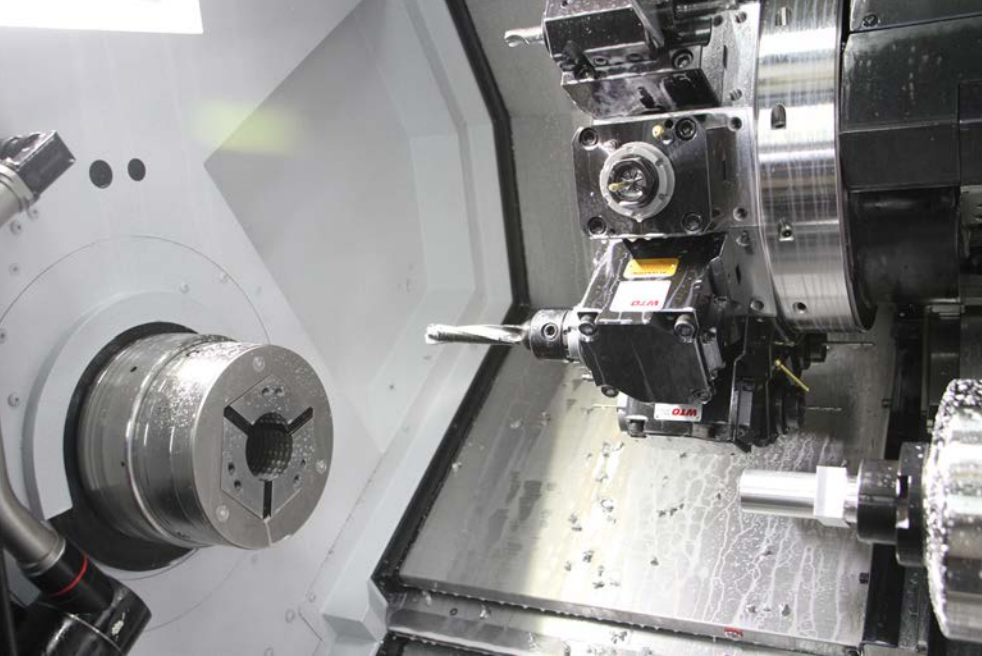
▲ A Hainbuch system is also used on the newly procured MoriSeiki NLX 2500 SY.
