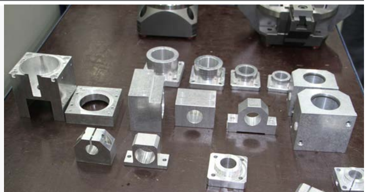
At Rodriguez a wide variety of linear technology components are manufactured on the Hermle C40.
