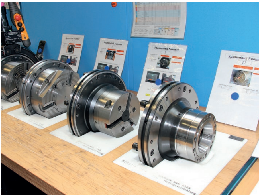
Pictured are: The different clamping devices with adapter plate that can be quickly mounted on the lathes.
