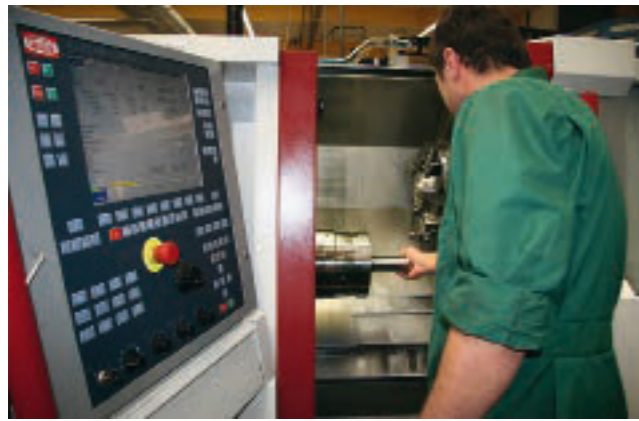
Mandrels and clamping heads can also be quickly and easily changed in the basic unit.
